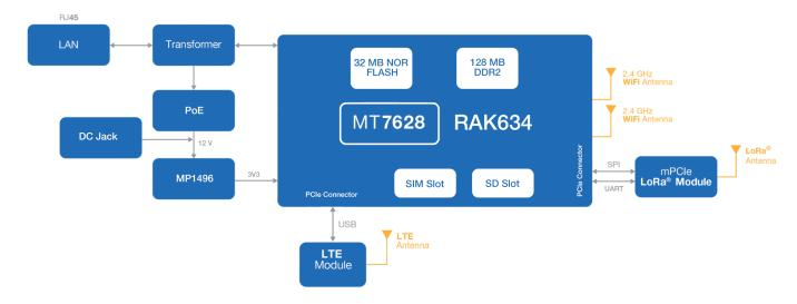
Figure 2: RAK7268V2 WisGate Edge Lite 2 with LTE Block Diagram
