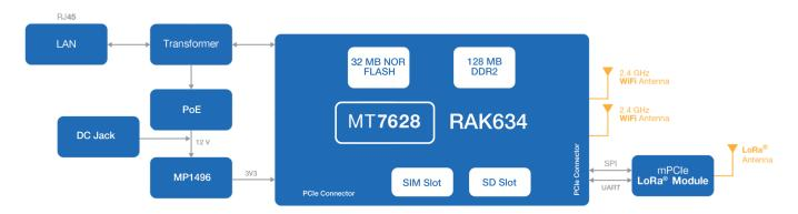
Figure 1: RAK7268V2 WisGate Edge Lite 2 without LTE Block Diagram
