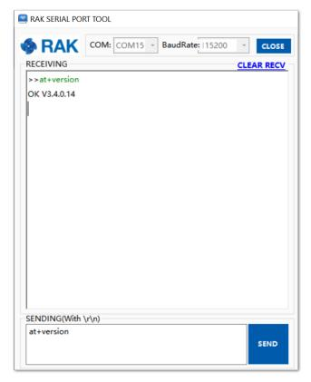
Figure 8: AT command for Firmware Version
