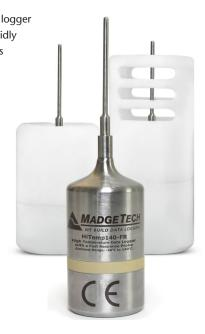
The Trigger Settings feature of the HiTemp140-FR allows users to configure high and low temperature thresholds that when met or exceeded, will automatically start or stop recording data to memory. This data logger is capable of storing up to 32,700 date and time stamped readings and features a nonvolatile solid state memory which retains data even if the battery becomes discharged.
