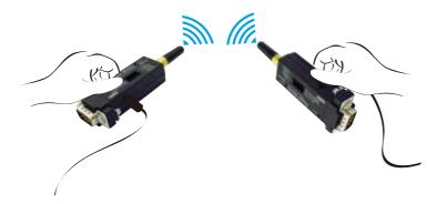
Parani-SD1100 provides Pairing Button for instant configuration without a PC to make an automatic connection between two Parani-SD1100s. In this example we will refer to the two Parani-SD1100s as SD1 and SD2. (Only single connection mode)
