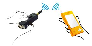
Using pairing button, users can make a pairing connection between a Parani-SD1100 and other Bluetooth devices. (Refer to the Parani-SD1100 as SD1)
