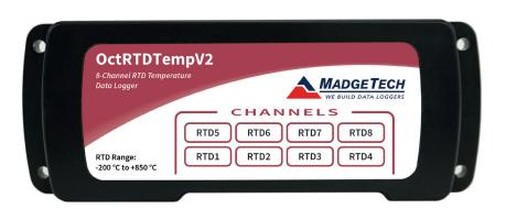
The OctRTDTempV2 is an 8-channel, RTD based temperature data logger with a reading rate of up to 4 Hz. It can measure and record up to 21,824 readings per channel. To maximize memory capacity, users can enable or disable channels. For easy identification, each channel can be named with up to a ten digit title. The storage medium is non-volatile solid state memory, providing maximum data security even if the battery becomes discharged. The OctRTDTempV2 makes data retrieval quick and easy.
