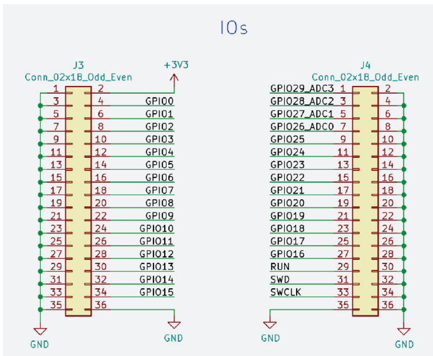
Figure 10. Schematic section showing the 2.54mm I/O headers
