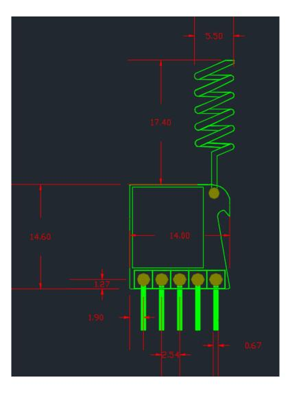
RYLR998 868/915MHz Lora Antenna Transceiver Module
