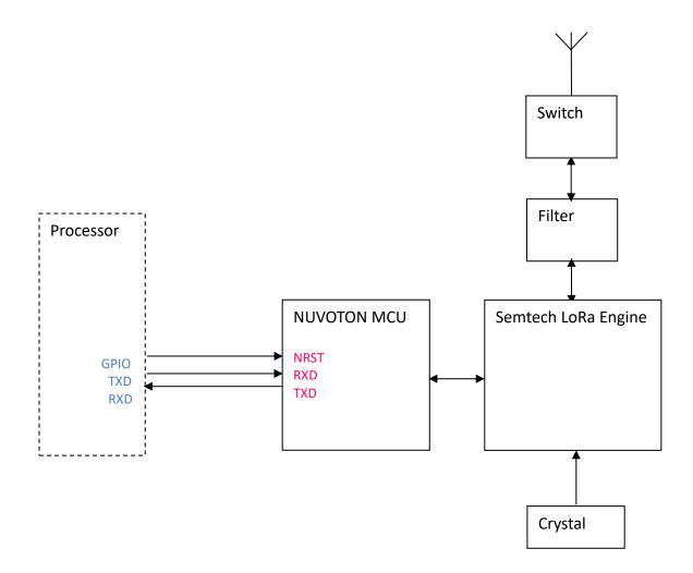
RYLR998 REYAX 868/915MHz Lora Antenna Transceiver Module
