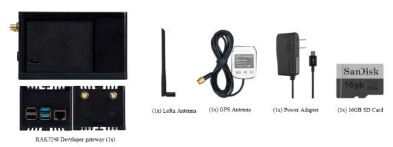
Figure 2: RAK7248/P WisGate Developer D4H Gateway package contents
