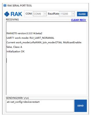
Figure 2: RAK Serial Port Tool Connected to RAK4270 Module
