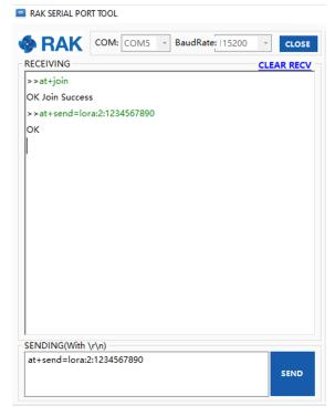
Figure 15: OTAA Test Sample Data Sent via RAK Serial Port Tool
