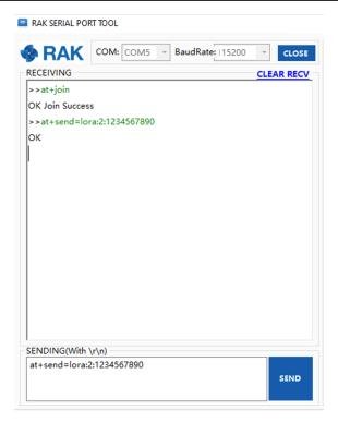
Figure 22: OTAA Test Sample Data Sent via RAK Serial Port Tool
