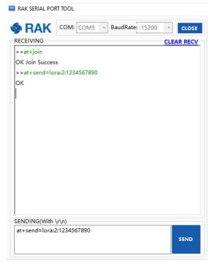
Figure 38: Chirpstack OTAA Join the Network via RAK Serial Port Tool
