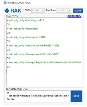
Figure 14: Configuring LoRa Parameters
