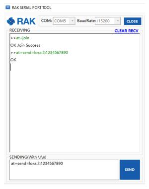
Figure 46: Chirpstack Sample Data Sent via RAK Serial Port Tool
