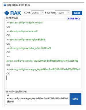
Figure 21: AT Command for ABP LoRa parameters via RAK Serial Port Tool
