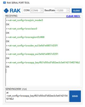
Figure 37: Chirpstack OTAA configuration via RAK Serial Port Tool
