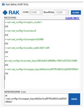
Figure 45: Chirpstack ABP Parameters Configuration via RAK Serial Port Tool
