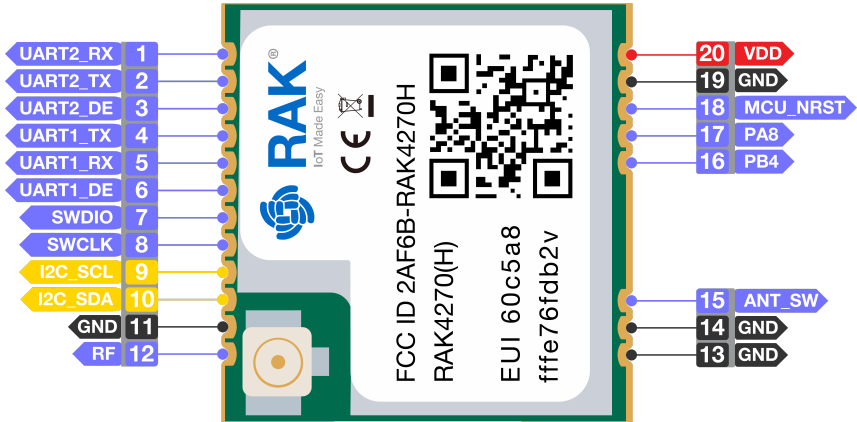
Figure 3: RAK4270 Pinout
