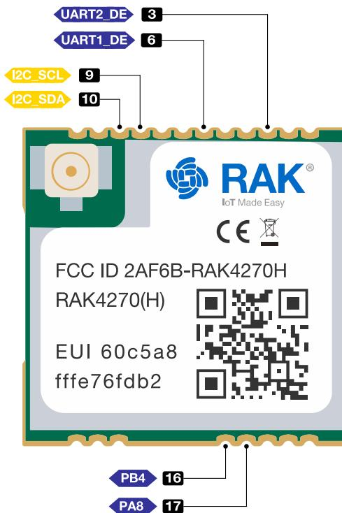
Figure 1: GPIO Pinout for RAK4270
